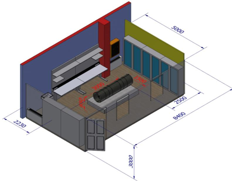
Figure 3: Rendering of the experimental hall for the FCC-ee IR mock-up in Building 5. The support tube, to be assembled in the final phase, is visible at the center.
