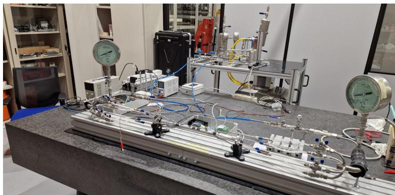
Figure 4: Experimental setup for thermal tests on the central beam pipe.
