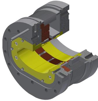
Figure 5: Proposed IR bellows with copper-beryllium RF fingers for electrical continuity, HOM absorber volume, and cooling pipe.
