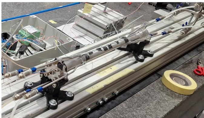
Figure 2: Full-scale aluminum prototype of the central beam pipe, used for initial thermal tests with water.
