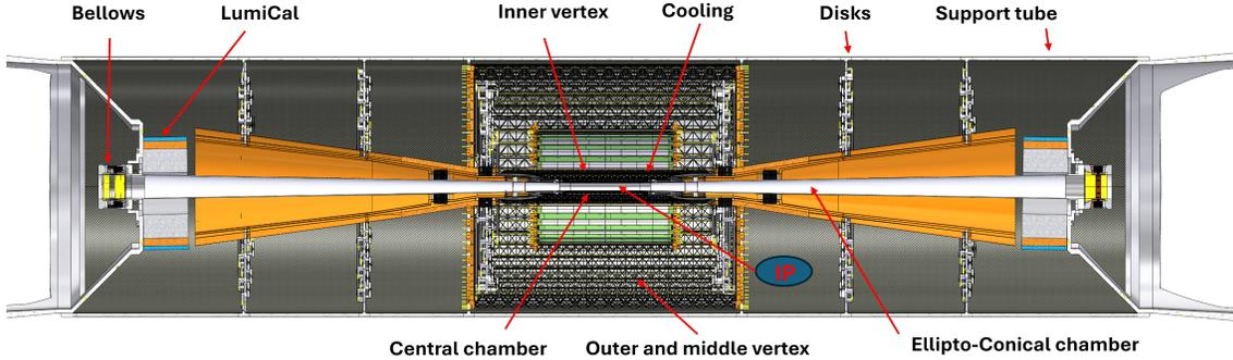
Figure 1: Machine-Detector Interface region of the FCC-ee, illustrating all elements to be assembled in the IR mock-up project.
